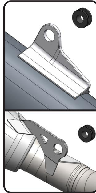
2. Install ALS-043, aluminum spacer into frontside and backside of Z1024, rubber grommets on muffler bracket and muffler chassis mount bracket.
