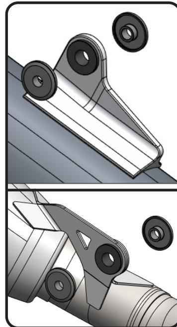
3. Install 23484-104, Yoshimura header using the stock header nuts. Do not torque at this time.
